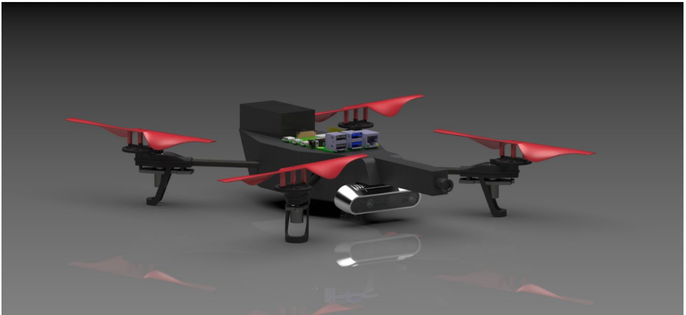
Figure 7: Final Drone Design: D435i Stereo Infrared Camera and Raspberry Pi 4
